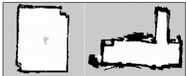
Fig. 15. Generated 2D Grid-Maps by RTAB-Map Algorithm
